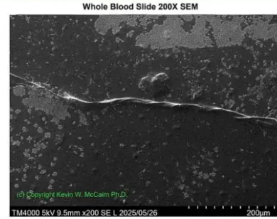
Figure 4. Scanning electron micrograph at 200X magnification. Fibrils show twisting, lamellar thickening, and increased density—hallmarks of mature amyloid filament aggregation.
